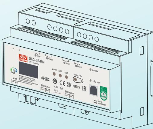
DLC-02-KN is a KNX to DALI gateway, used to connect a digital DALI lighting system to the KNX installation. Room-based lighting control is conveniently incorporated into the higher-level KNX system building management system. The device transforms switch and dim commands from the connected KNX system into DALI telegrams and status information from the DALI bus into KNX telegrams.
