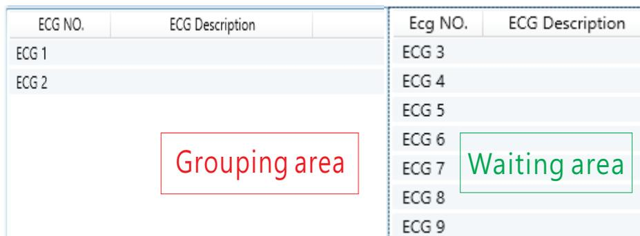
( 3 ) After grouping, please click on the "Partial download" or "Full download" button to download the grouping information to the gateway and ECGs. After downloading, click the right mouse button to perform lamp on, lamp off, and flashing tests on the group.
