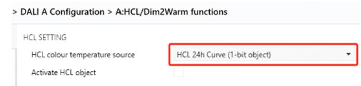
Step 3: On the "A: HCL 24-hour Curve" page, set the 24-hour colour temperature curve as shown in the following figure.
