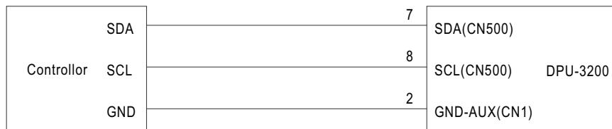
3. Communication function can be accessed immediately after DPU-3200 is connected to AC. Set output voltage at 56V.
