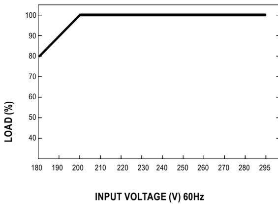
※ De-rating is needed under low input voltage.
