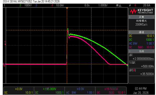
INPUT=230VAC/50HZ @ FULL LOAD CH2 : AC Input Voltage CH4 : Input current
