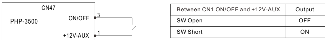
Figure 3-3 Connection of Remote Control
